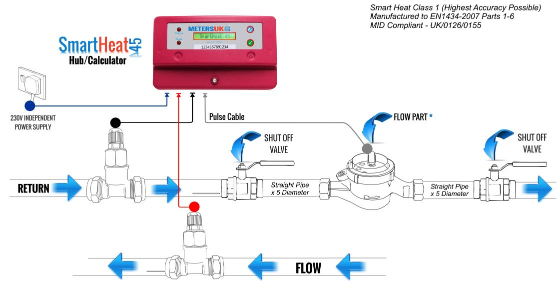
\*\* Heating System: The flow part is recommended to be installed in the RETURN pipe Cooling System: The flow part is recommended to be installed in the FLOW pipe
