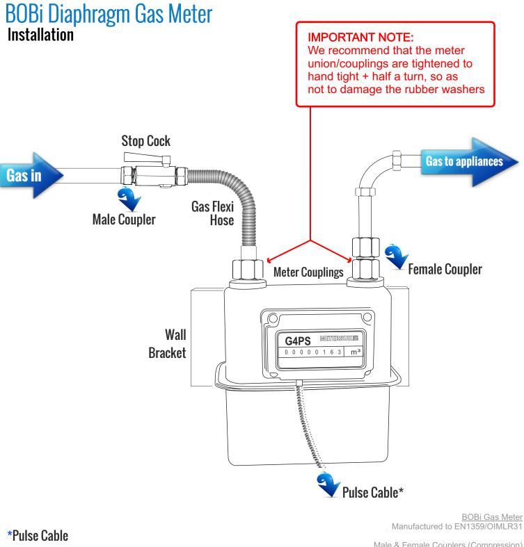
If you are not using the gas meter for remote reading you will not need to use the pulse cable.
