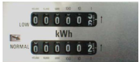
Single Rate 6 figure cyclometer with quick-change number and transfer mechanism
